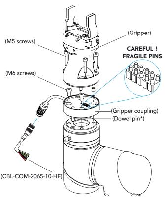
\*The dowel pin is meant to have a tight fit on the robot side and a slip fit on the effector side of the assembly.
