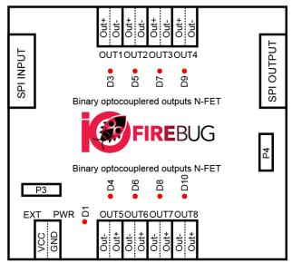
SPI INPUT allows to connect with the IOFireBug Engine or with previous expansion module. SPI OUTPUT allows to connect following expansion module. Closed jumper P5 defines that current Wagon 16I is the last connected module in IOFireBug Engine configuration (in other words, there is no following expansion module connected to SPI OUTPUT).
