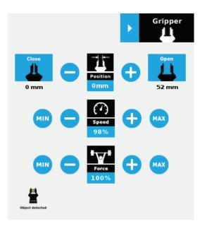
• Depending on the PolyScope settings used, the Gripper position measurements can either display in metric or imperial units.
