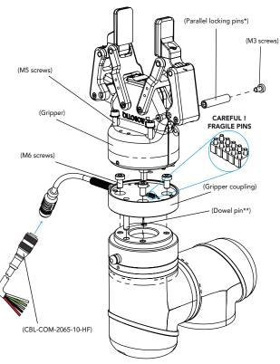
\*Parallel locking pins can be installed to perform exclusively parallel grasps with the Gripper. See instruction manual for more details.
