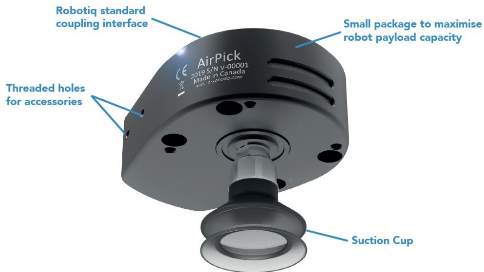
Fig. 1-1: Robotiq AirPick Gripper
