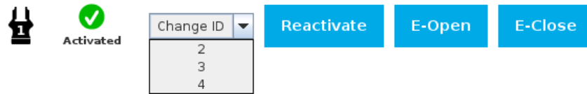
Fig. 4-15: Gripper ID modification in the Gripper Dashboard
