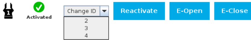
Fig. 4-17: Gripper ID modification in the Gripper Dashboard
